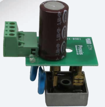
3300 µF KONDANSATÖRLÜ KÖPRÜ DİYOT KARTI (35A) BRIDGE DIODE CARD WITH 3300 µF CAPACITOR (35A)
