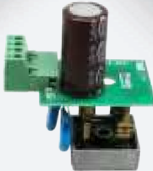
3300 µF KONDANSATÖRLÜ KÖPRÜ DİYOT KARTI (35A) BRIDGE DIODE CARD WITH 3300 µF CAPACITOR (35A)
